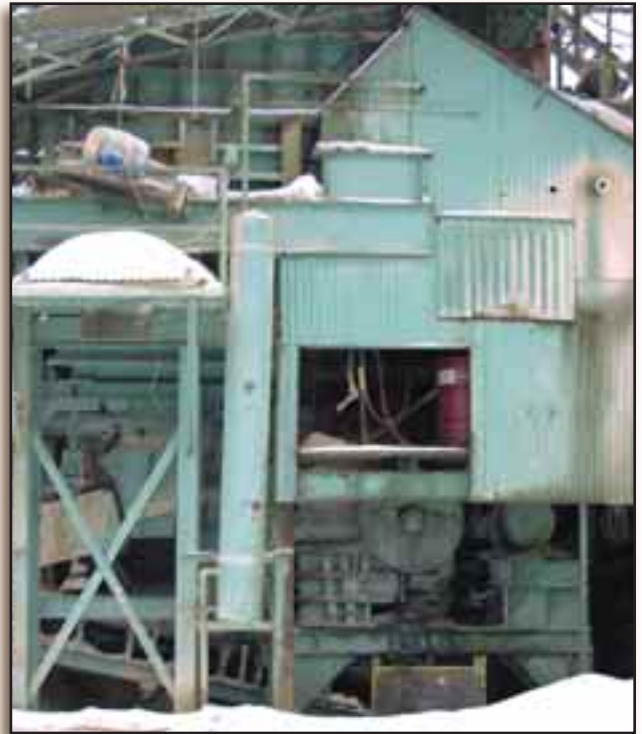
This Pioneer 2036 Jaw, built in 1938, is still running at the Sharon Conglomerate sandstone deposit near Chardon, Ohio. Production rates for the primary jaw are 200 to 225 TPH in abrasive silica sandstone.
