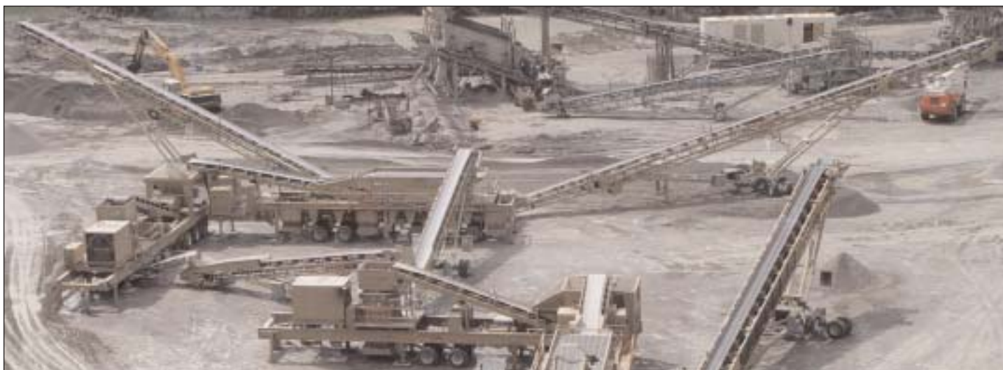
The “back half” of Whitaker Contracting’s Fast Pack Plant consists of a second JCI 8203 horizontal screen, Kolberg Series 11 stacking conveyors and a second JCI K400 Cone Crusher. The sized material coming from the second cone recirculates to the second 8203 screen. In this picture, the first K400 cone is visible in the foreground.
