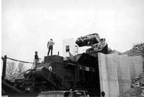
Material is fed to a portable Pioneer 4654 Horizontal Shaft Impactor where a vibrating grizzly separates the material.
