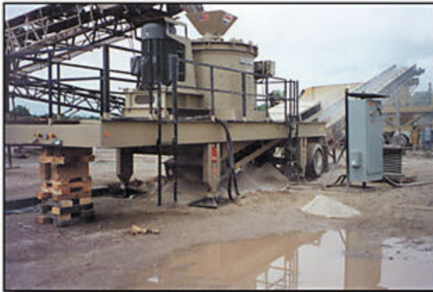
The 2500 VSI gives us the shape of aggregate we need to meet superpave specifications.
