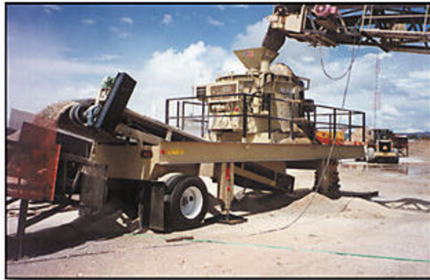
Associated Asphalt Materials' Espanola, NM, crushing plant spread showing the Pioneer 2500 Ultra-Spec VSI. Owner Richard Cook purchased the 2500 Ultra-Spec VSI in order to meet New Mexico's Superpave specifications.
