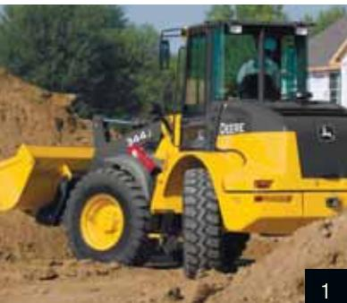
1. Unique stereo steering turns tighter while actually articulating less to provide superior close-quarters maneuverability.
