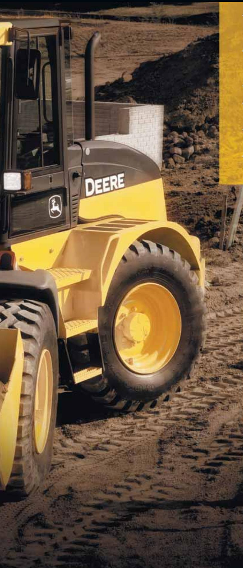
A 20-percent tighter turning radius allows the 344J to work where comparable loaders won't — for maximum productivity in close quarters.
