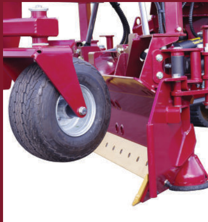
Hydraulic wings control material in both directions
