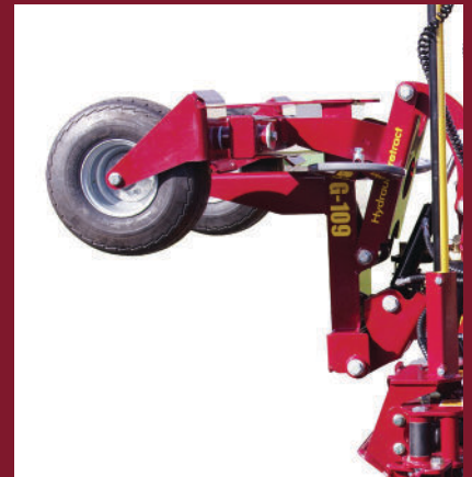
Retracting front chassis gets into corners
