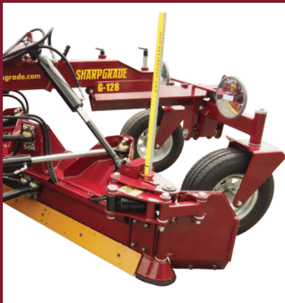
Rear blade to precision grade in reverse
