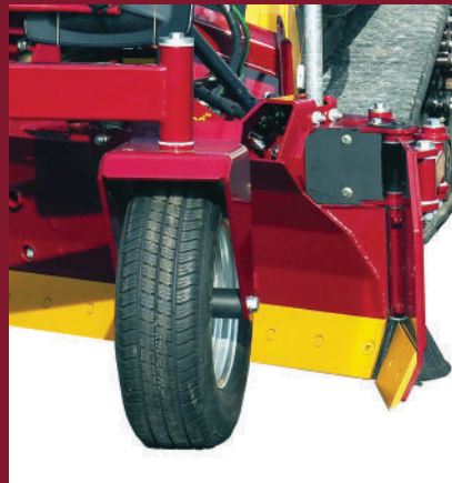
Hydraulic wings control material in both directions
