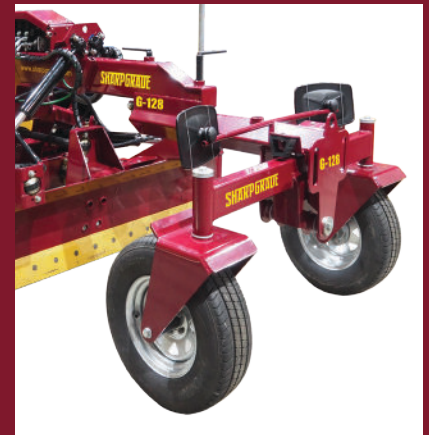
Telescopic retracting wheels for confined space / transport
