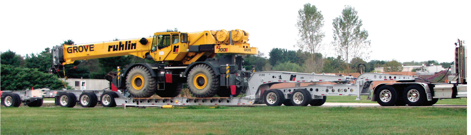
RTN55TD3-R4A Hydraulic Booster Axle and Deck Extension
