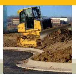
Infinitely variable track control lets you speed up or slow power to either track, delivering smooth, full-power turns that don't rob horsepower or tear up soft terrain.
