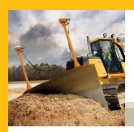
Equipped with optional Intergrated Grade Control (IGC) package, your dozer arrives from the factory "plug and play" ready. Open architecture design lets you employ the electronic grade-control system that's right for you.
