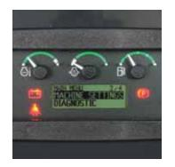
Customizing machine operation is push-button easy through the monitor. TMC monitor lets you fine-tune decelerator mode and response, forward/reverse ground speed ranges, steering modulation, and forward/reverse speed ratios. For unmatched control.
