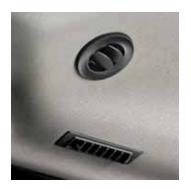
Automotive-style directional vents help keep the view clear, while delivering warm or cool air quietly and efficiently. Air conditioning is standard on all cabs. An optional under-seat heater is available for non-cab crawlers.
