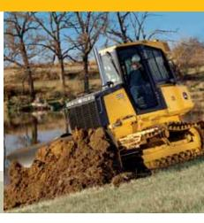
The 700J steers the same and maintains its preset speed whether it's on level ground or a 2-to-1 slope. For total control regardless of the terrain.
