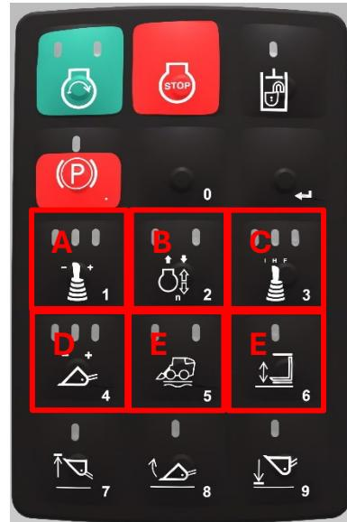
**A: Transmission Response (Optional): EH machines only, if equipped with joystick performance package.**
