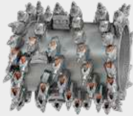
Standard Milling Drum Milling width: 3 ft 3 in (1,000 mm) Milling depth: 0 to 13 in (0 to 330 mm) Tool spacing: 0.6 in (15 mm)
