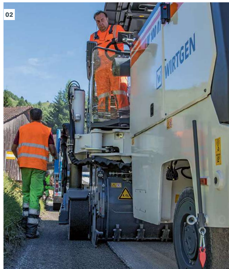
01 The camera's ability to see and display key work areas enhances performance and quality. 02 The operator always has an unobstructed view of the right side plate.
