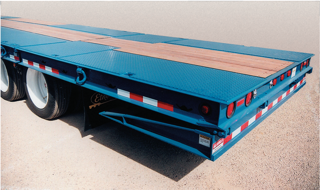
Etnyre custom designed tiedowns and optional stake pockets.
